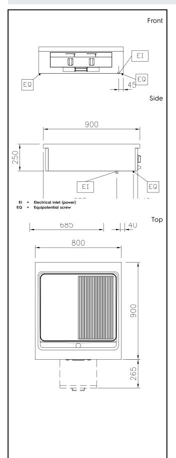
Electric Supply voltage: 440 V/3 ph/50/60 Hz Total Watts: 15.3 kW **Key Information:** Cooking Surface Depth: 615 mm Cooking Surface Width: 700 mm 80 °C Working Temperature MIN: 280 °C Working Temperature MAX: External dimensions, Width: 800 mm External dimensions, Depth: 900 mm External dimensions, Height: 250 mm Net weight: 120 kg Configuration: One-Side Operated;Top Cooking surface type: half ribbed/ half smooth Chromium Plated mild steel Cooking surface - material: mirror
